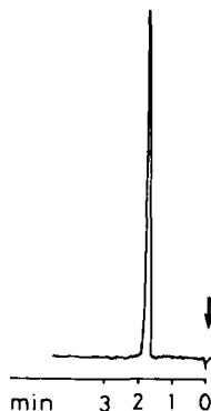
FIGURE 3. Chromatogram of lithium, retained as ion pair with octyl sulfate. Solid phase: LiChrosorb RP-18, 10 \mu m; Eluent: 0.005 M octyl sulfate in phosphate buffer pH 3.0 with 1.15% 1-pentanol; Flow rate: 1.3 ml/min; Detector: flame photometer; Sample: lithium (0.2 \mu g).
